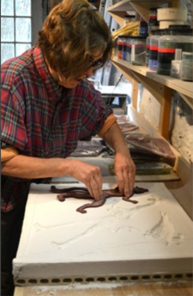
(Above) Two clay figures for Allegra's Jazz Band lie top down. Notice the little protrusions that Allegra holds when (below left) she presses the figures down into dry plaster. This action (below right) results in a kiln-ready mold for the glass.
