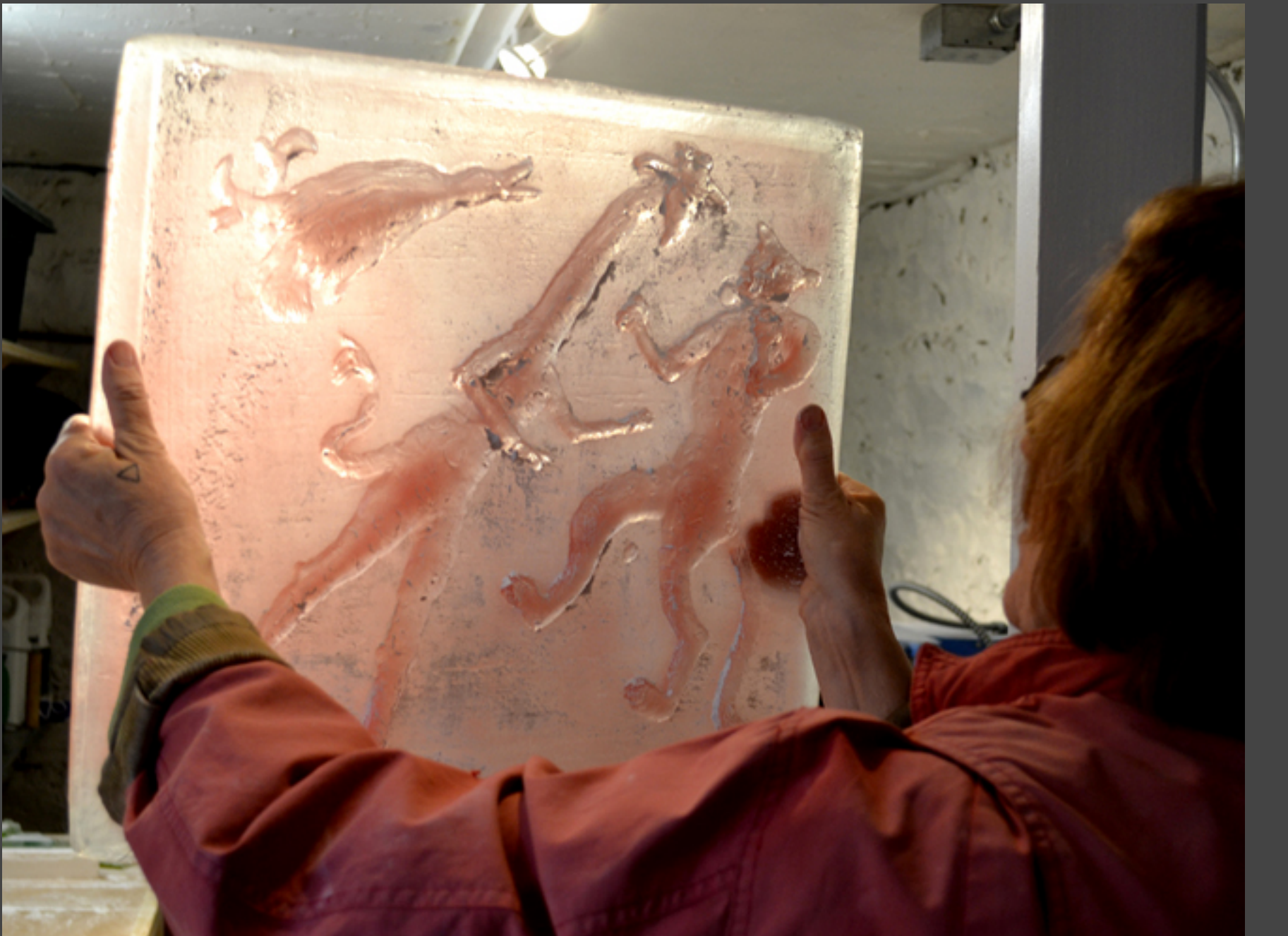
(Above) The dry plaster mold (contained in fiber board) rests half in the kiln. Then Allegra places glass on top and slides it into the kiln. (Below) After firing, Allegra inspects the panel.
