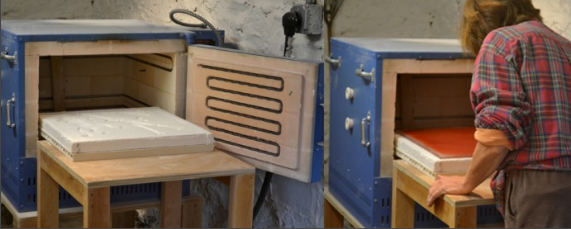
(Above) The dry plaster mold (contained in fiber board) rests half in the kiln. Then Allegra places glass on top and slides it into the kiln. (Below) After firing, Allegra inspects the panel.
